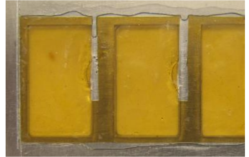
Flexible wall material “EP-0.5” (thickness 0.5mm)
